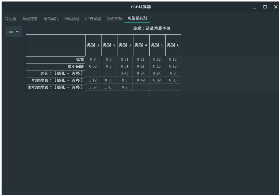
The screenshot shows the 'PCB计算器' (PCB Calculator) application window. The '电路板类别' (PCB Category) tab is selected. A dropdown menu is set to 'mm'. A warning message reads '注意：该值为最小值' (Attention: This value is the minimum). The table below lists the minimum values for various parameters across six categories.
